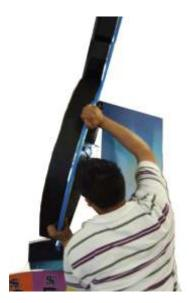
3. Connect the following: wheel motor cable, marquee cables, wheel LED lamp cables and cabinet speaker cables to their mates in the back of the main cabinet. Verify secure connections.
